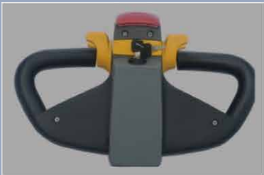
Key switch and meter are integrated in the handle
